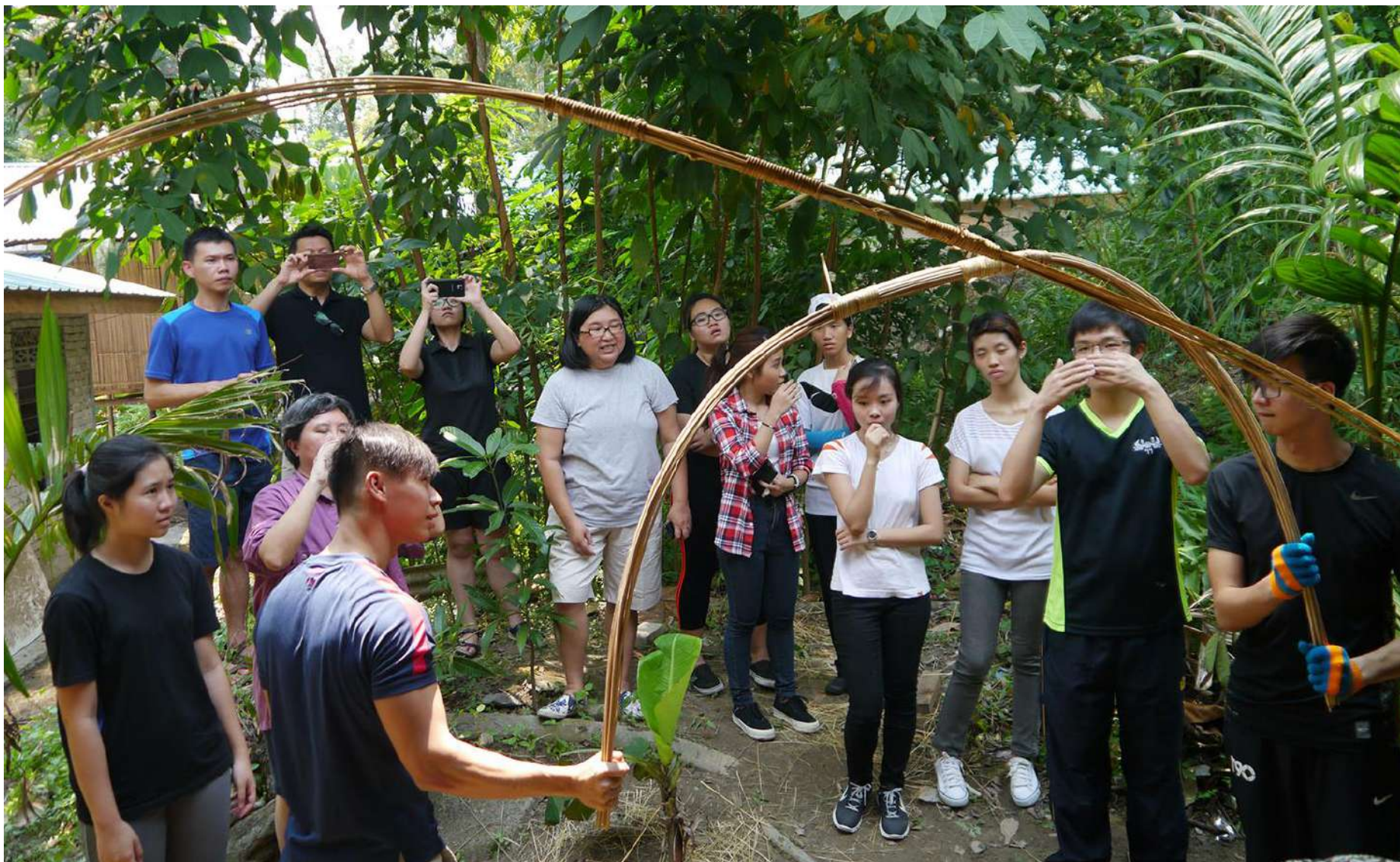
The strength and flexibility of the students' finished 10m bamboo bundle is tested against Raman's 5m bundle. It was decided that the bamboo sections in the students' 10m bundle were cut too thin and that next time, they should be made thicker to make the bundle stronger.
