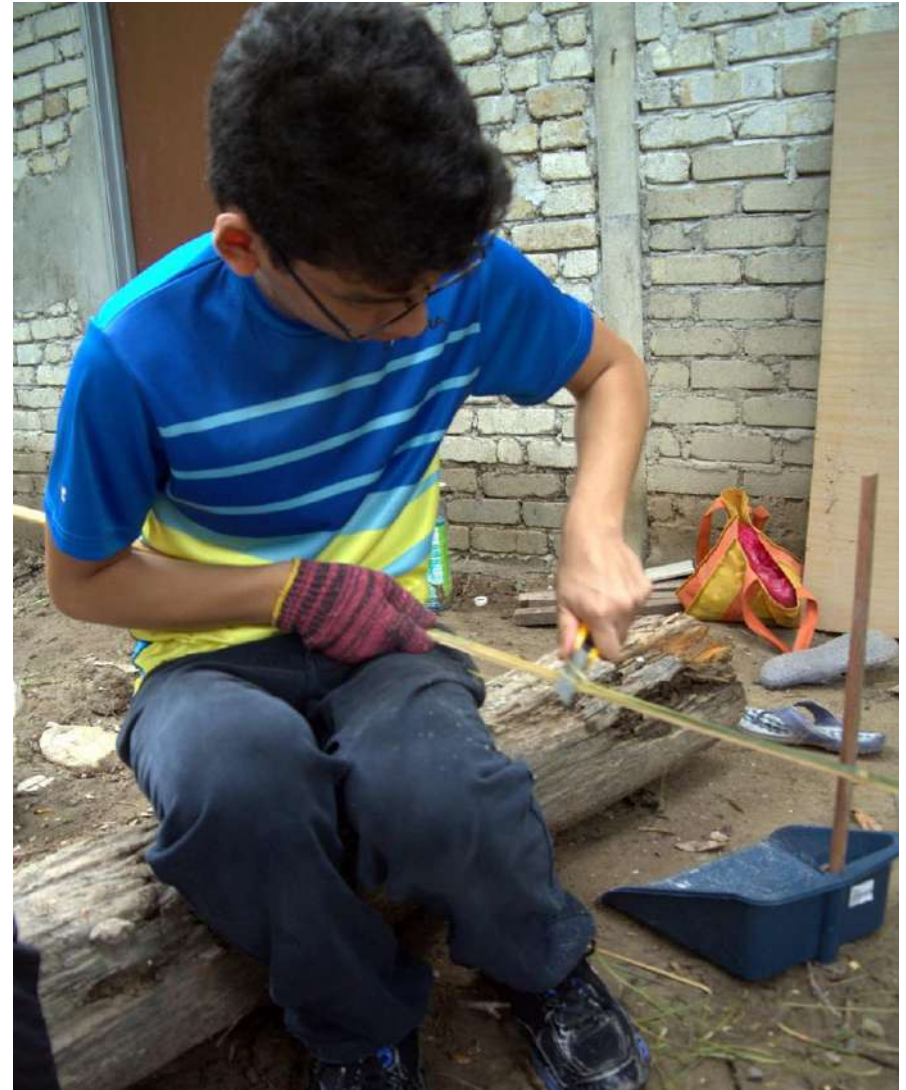
A Taylor's student in the process of rounding down the raw bamboo sections' edges.
