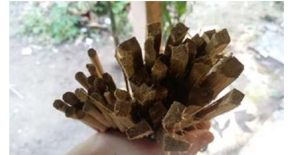
Raw sections of a bamboo culm after it has been split into segments.
